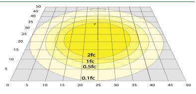
Simulation Based on 4000K Area 50'x 50' Mounting Height: 9'
